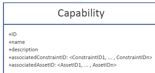
Figure 13: UML representation for Capability modelling
